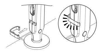
INSTALLATION OF LOCKING PLATE KIT COMPLETE
